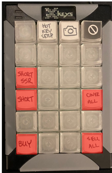
Figure D.3 - X-keys macropad used to execute hotkeys with one button.
